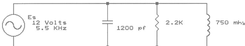
Resonant Frequency = \_\_\_\_\_ Hz
