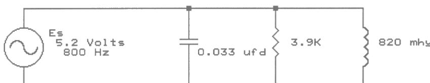
Resonant Frequency = \_\_\_\_\_ Hz
