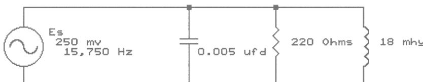
Resonant Frequency = \_\_\_\_\_ Hz
